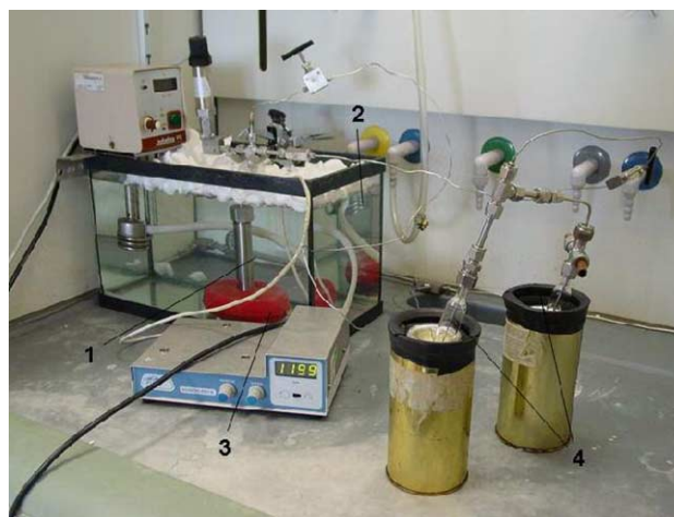
Fig. 1. Apparatus used for supercritical CO 2 extraction: high pressure cell (1), water bath (2), mixing plate (3), cold traps (4).
